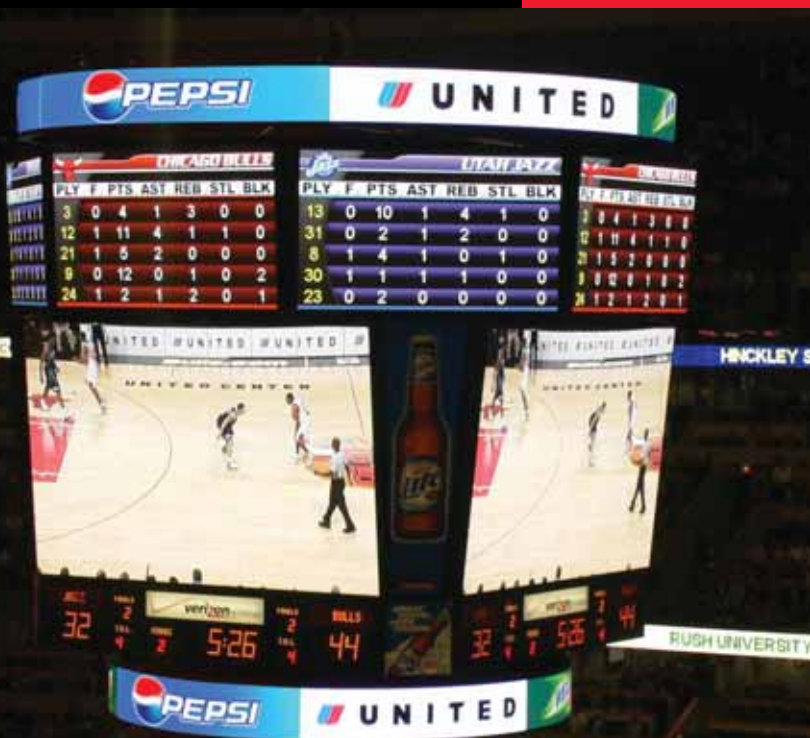
United Center, Chicago: 3.901m x 6.178m 4 sets, 2.276m x3.901m x 8sets 5mm Dot Pitch.
