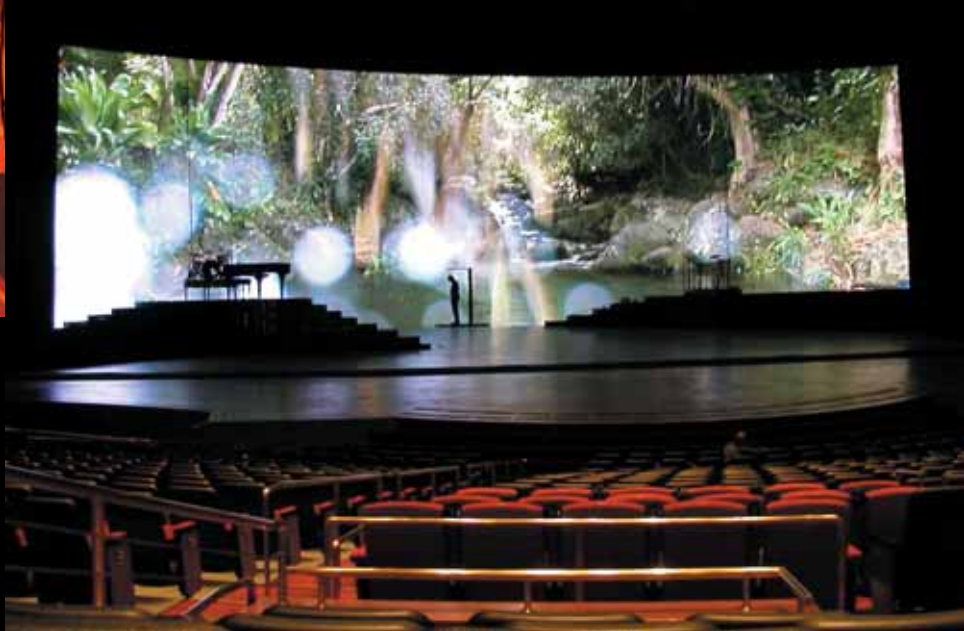
Colosseum at Caesars Palace, Las Vegas: 10.24m x 33.28m, 8mm Dot Pitch.
